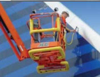
The Model 740AJ is capable of reaching all external surfaces on any aircraft manufactured today, even the 747 and military C5B.
