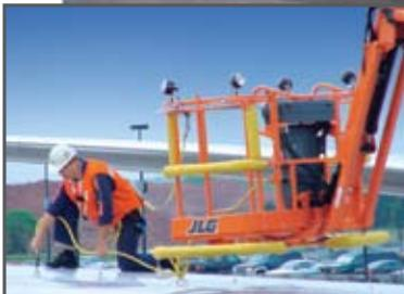
The optional Soft Touch System reduces the risk of accidental contact and damage during aircraft maintenance. This optional package features a suspended padded rail that surrounds the platform basket. Proximity sensors de-activate platform movement functions and alert the operator if the basket comes too close to the aircraft surface.
