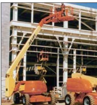
Jib-equipped models add 70 degrees of upward and 60 degrees of downward motion.
