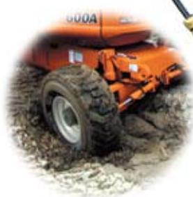
Four-wheel drive option and a standard oscillating axle provides superior terrainability.
